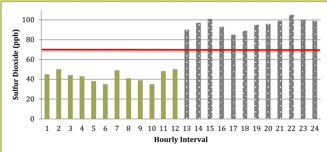
**Figure 6. Sample US EPA Ambient Air Quality Monitoring of Sulfur Dioxide (1-hour mean)**
